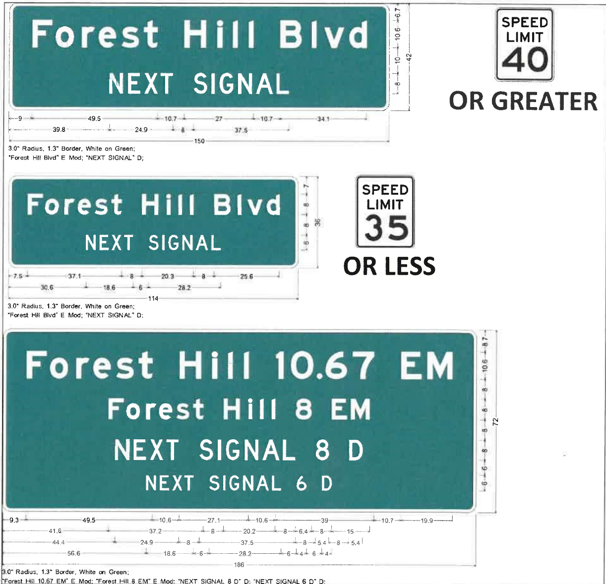
Figure 18 – 1 Examples of Advance Street Name Signs
